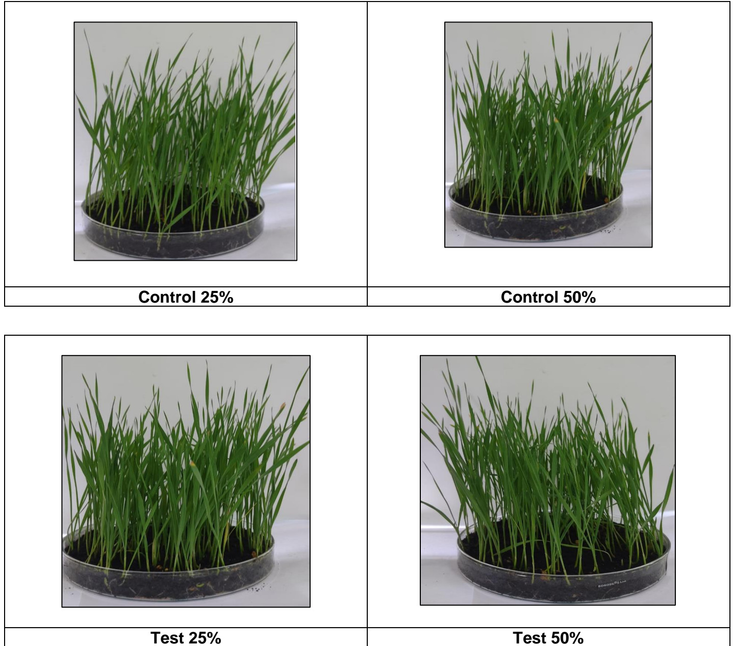
Figure 4: Effect of compost Molded Fiber Coffee Cup Lids on Triticum aestivum growth
